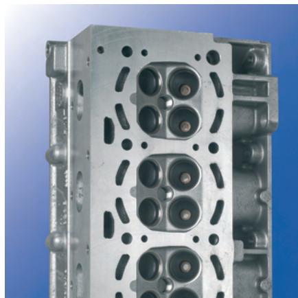
Demanding: Complete machining of a cylinder head
